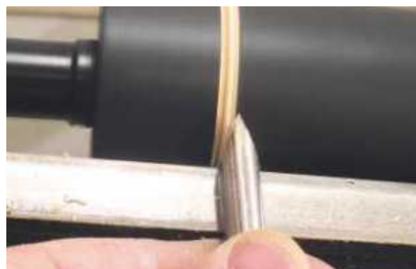
▲ Pic.20 The round skew has a few advantages; it'll make a 'V' just as you can with the ordinary version, although I also find it easier to sharpen
